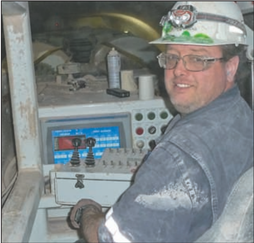
Richard Cozens is a Journeyman Miner Operator at the Rocanville site. After a 45 minute truck ride to his mining site, Cozens uses a laser, gauges on his machine, his eye and intuition to guide the giant miner. The machine has four giant discs with metal teeth on them that grind the front of the wall. The crushed ore is then channelled towards a conveyor belt that moves it to hoppers before it is shot to the surface 3500 feet above. Two workers join Cozens at his machine and they are kept busy adding conveyor belt posts and stringing plastic that helps direct air. There are literally hundreds of miles of conveyor belts in these mines.
